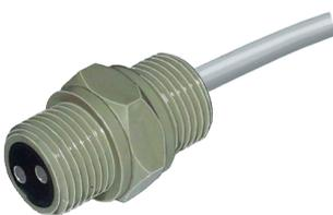
The electrode NE2 with its 1/2" thread can directly be screwed into the wall of a tank. The two electrodes (stainless steel V4A) are flush cast in a plastic housing (Polypropylen, PP) with cast resin. The electrode can be used in a temperature-range -5...+60 °C and is pressure-resistant up to 6 bar. The ingrained cable with 2 strands, each 0,25 mm<sup>2</sup>, is 2000 mm long,  $\varnothing$  4 mm.
